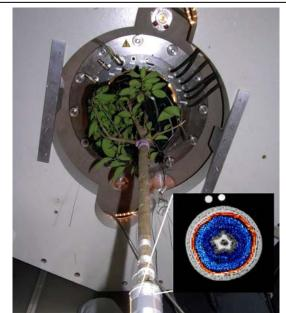
With MRI on intact plants the transport of water in the stem can be monitored directly and non-invasively. The inset shows a slice trough the stem, coloured according to flow properties.
