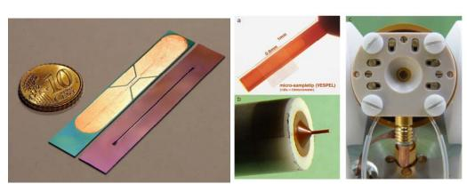
New miniaturized NMR detector technologies open the way for detection of nanoliter volumes. In the liquid-state the stripline detector (left) allows in-situ reaction monitoring in microfluidic devices, whereas the piggy-back magic angle spinning device (right) opens the way for high-resolution solid-state NMR of micro crystals. Ongoing research at the Radboud University Nijmegen.
